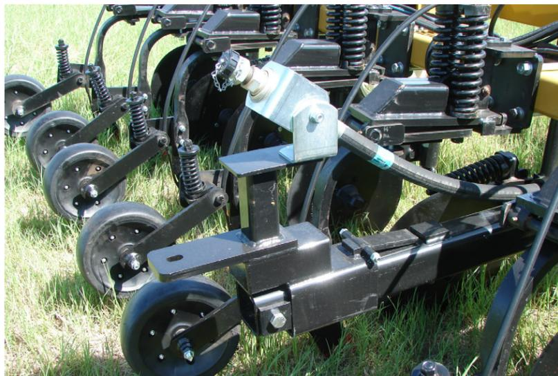
**HEAVY DUTY, SPRING LOADED, SWIVELING COULTER
