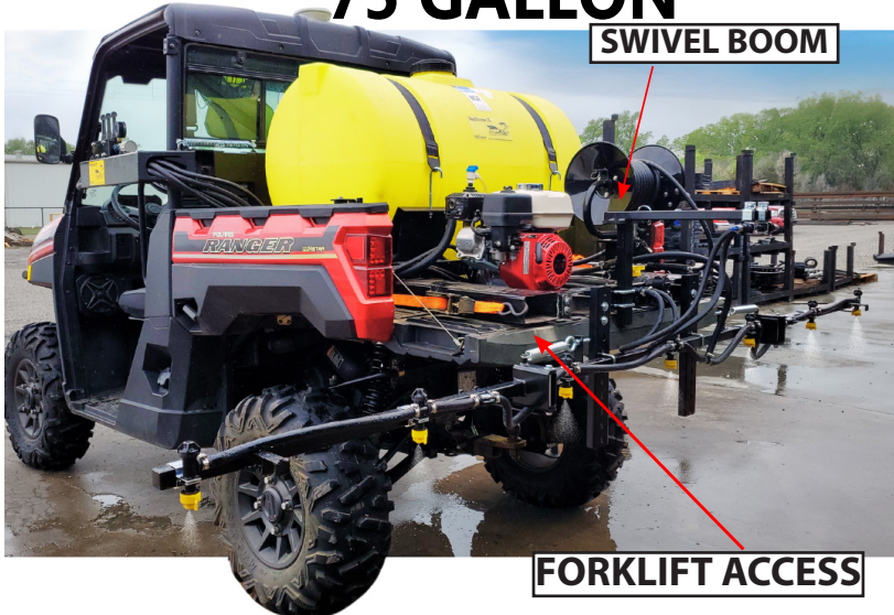
PICTURED: GAS POWERED WITH 12' BOOMS AND BOOMLESS NOZZLES
